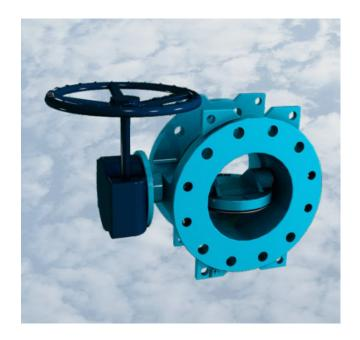
VOSA double eccentric butterfly valves are designed for installation in water supply systems to enable isolation of water lines and come standard with flanged end connections. The standard valve incorporates a rubber seal ring that is retained on the valve disc (SEAL ON DISC design) and is manufactured using VOSA drinking water approved EPDM rubber and is offset to the disc shaft centreline – so the shaft does not pass through the seal.
