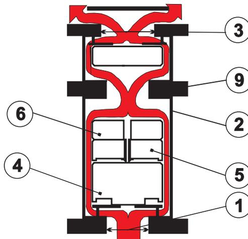
Air enters Orifice (1), travels through the annular space between the cylindrical floats (4) , (5), (6) and discharges through the Large Orifice (3) into atmosphere.\*
