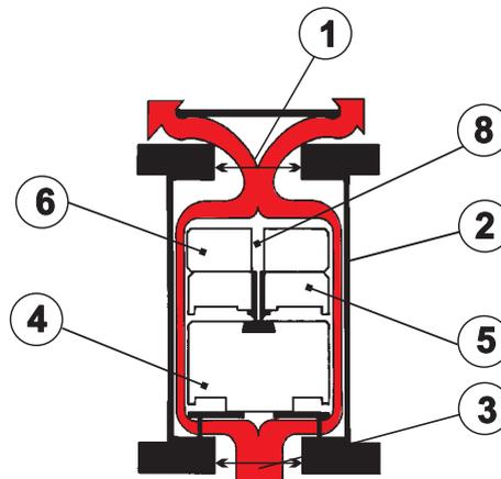
Air enters Orifice (3), travels through the annular space between the cylindrical floats (4), (5), and (6) and the valve Chamber Barrel (2) and discharges from the Large Orifice (1) into atmosphere.
