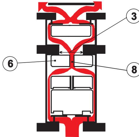
In reaction to increased air flow, Float (6) closes Large Orifice and air is forced through the "Anti-Shock" Orifice resulting in deceleration of the approaching water due to the resistance of rising air pressure in the valve.
