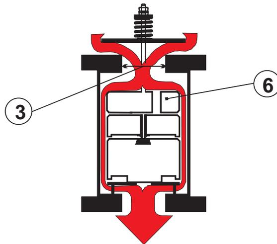
Upon pump stop, the pump discharge check valve closes. Liquid drains from the air valve and the pump's vertical column. The negative differential created by the draining liquid causes atmospheric air to push the "Anti-Shock" Float (6) down, opening the Large Orifice (3) and rapidly displaces the draining liquid to prevent potentially damaging internal negative pressure \*.
