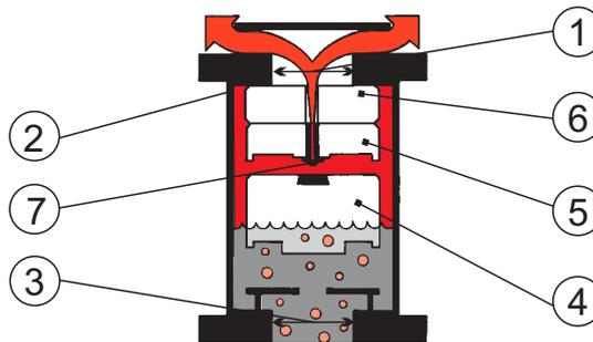
Subsequent to the filling of a pipeline, liquid enters the valve Barrel Chamber (2) and the Floats (4), (5) and (6) are buoyed so that the Large Orifice (1) is closed by Float (6), the valve will then become internally pressurized. A minimal working pressure of < 0.5 bar acting on the relatively large area of the Orifice (1) will lock Float (6) into the closed position across the Large Orifice (1).
