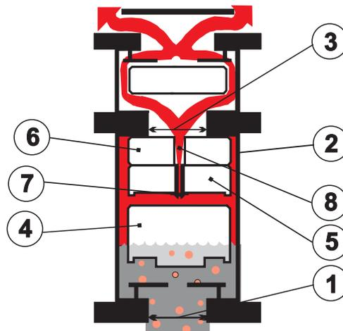
Subsequent to the filling of a pipeline, liquid enters the valve Barrel Chamber (2) and the Floats (4), (5) and (6) are buoyed so that the "Anti-Shock" Orifice (8) is closed by the Float (5) and the valve will then become pressurized. A minimal working pressure of <math><0.5\text{ bar}</math> acting on a relatively large area of the Orifice (1) will lock Floats (5) and (6) into the closed position across the Large Orifice (3).
